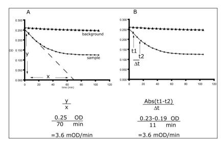
**A**: The rate is determined by calculating the gradient of the initial slope over the linear region.
